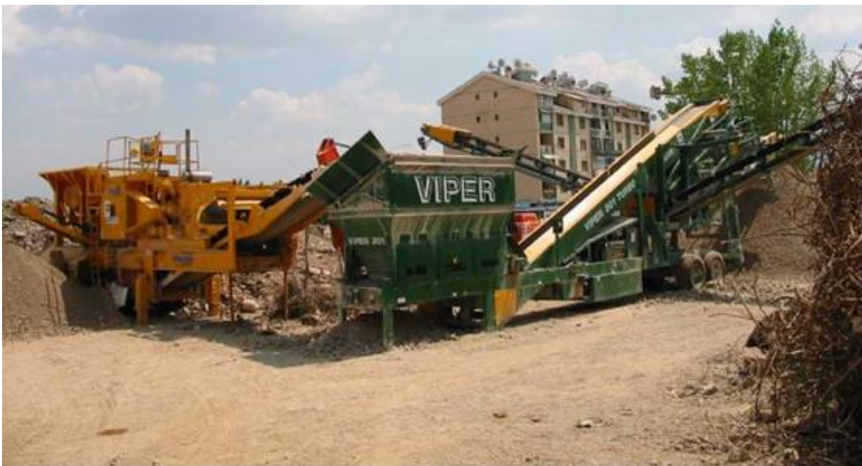
Figure 6: Example mobile debris recycling plant deployed in Kosovo 10 for processing the urban demolition waste and debris.
